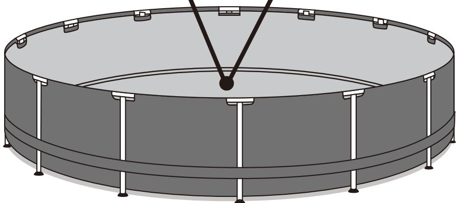
**EN** After the installation of the pool's steel frame is completed, ensure that the verticals are perpendicular to the ground. If they aren't, the verticals could be bent or deformed.
