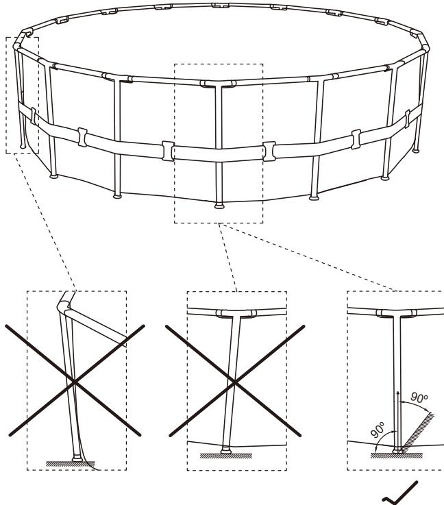
**EN** Do not assemble with pool legs on soft lawn. If you must assemble the pool on a soft surface, timber boards (not included) must be placed under the feet of the vertical support rods for even weight distribution.
